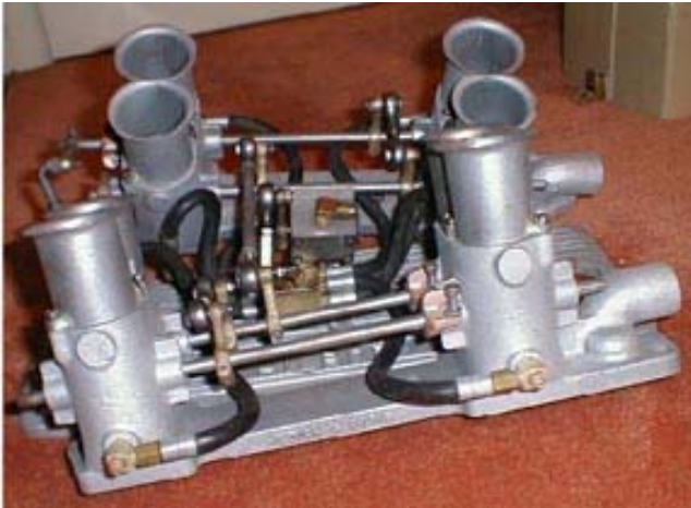
Another view of the Hilborn. Note that all 8 throttle plates are connected to shafts, which are operated off a bellcrank. All 8 throttle plates open and close together.
