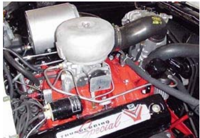
Another view of the supercharged Y. Note the bonnet and ducting from the compressor. Also note the filter housing behind the bonnet.
