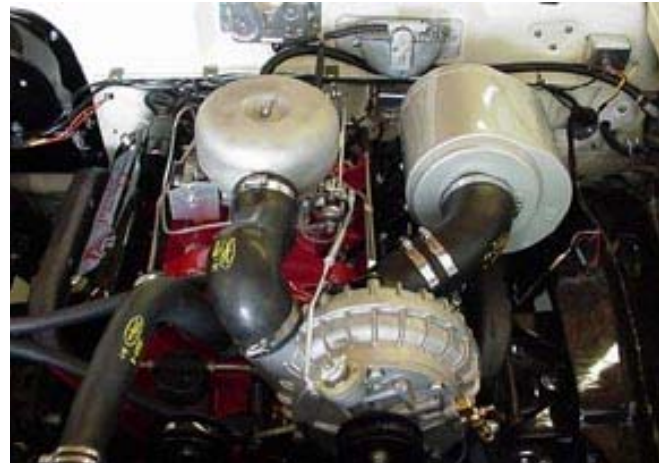
This is a McCulloch supercharger setup. We know them now as Paxton, and these have powered many a Ford to impressive times at the track.
