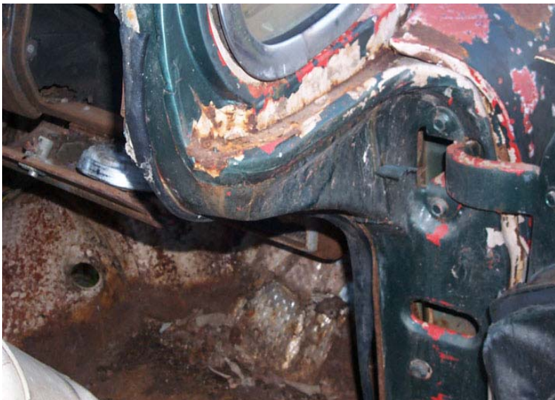
Doglegs are great shape. Hinges are still tight.
