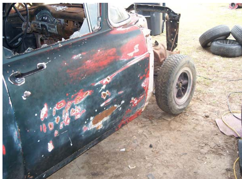
You can see the nice radiator support still attached with round rod to the front frame section. Rockers are fine also.
