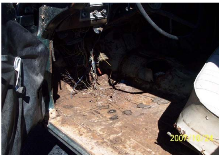
Check out the cool stretched naugahyde door panel. Any bidders? Holes in floor and tunnel are the worst damage.
