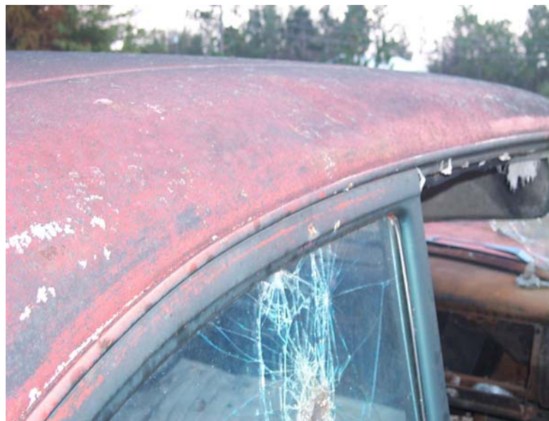
Note the big dent above the B-pillar, and the vinyl glue.
